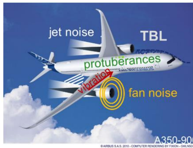
Figure 14. Sources of interior noise prediction [13]
