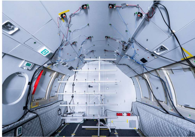
Figure 5. Disposition of microphones and actuators in an aircraft to perform global ASAC [14].
